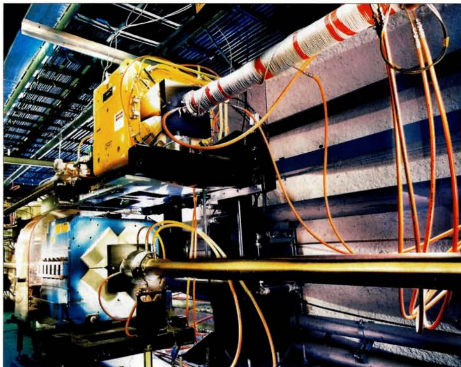
The PEP-II facility, with the positron ring above and the electron ring below. (Courtesy SLAC.)
