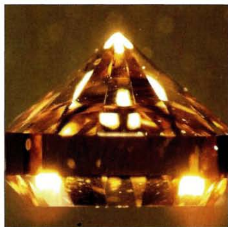
A synthetic-cut single-crystal diamond, about 2.5 mm high, grown by chemical-vapour deposition at the Carnegie Institute. The team at Carnegie have found that these diamonds are the hardest yet. (Photo courtesy of Physica Status Solidi.)
