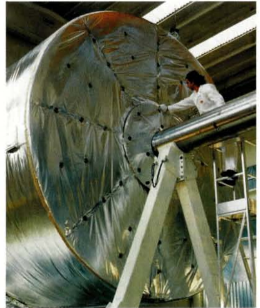
VIEW OF ENDCAP CRYOSTAT AND INTERNAL SUPER-INSULATION TEST ON SUPER-INSULATION PERFORMANCE: < 1 \text{W/m}^2
