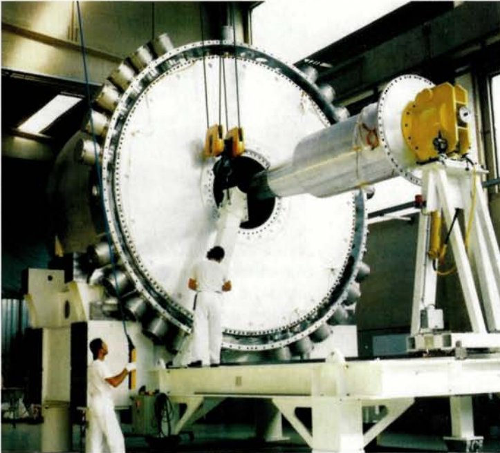
ENDCAP CRYOSTAT FOR ATLAS EXPERIMENT/LHC PROJECT MATERIAL: ALUMINIUM AL 5083; THICKNESS: 160 mm; EXT. DIAM. 5.500 mm; HEIGHT: 3.700 mm; WEIGHT 30.000 Kg; TESTS: HYDRAULIC TEST, CRYOGENIC TEST: 90K He Leak Test ( < 1 \times 10^{-8} mbar.l/s)
