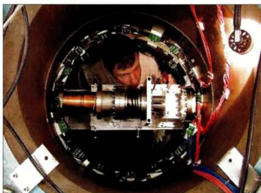
MISTRAL's new RF modulator is mounted so that the ^{11}\text{Li} experiment can be performed.
